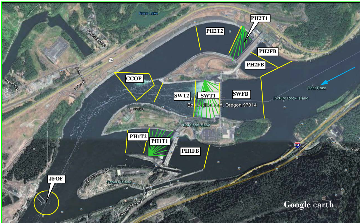
Figure 4. Zone map of Bonneville Dam used in 2012. Yellow lines delineate the zones, green lines represent the avian deterrent lines (not exact number), and the blue arrow indicates flow direction.
